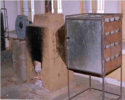
Waste fired dryer
